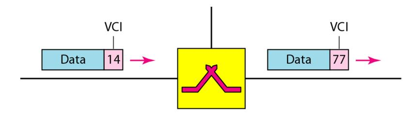
Figure 8.12 Switch and tables in a virtual-circuit network
