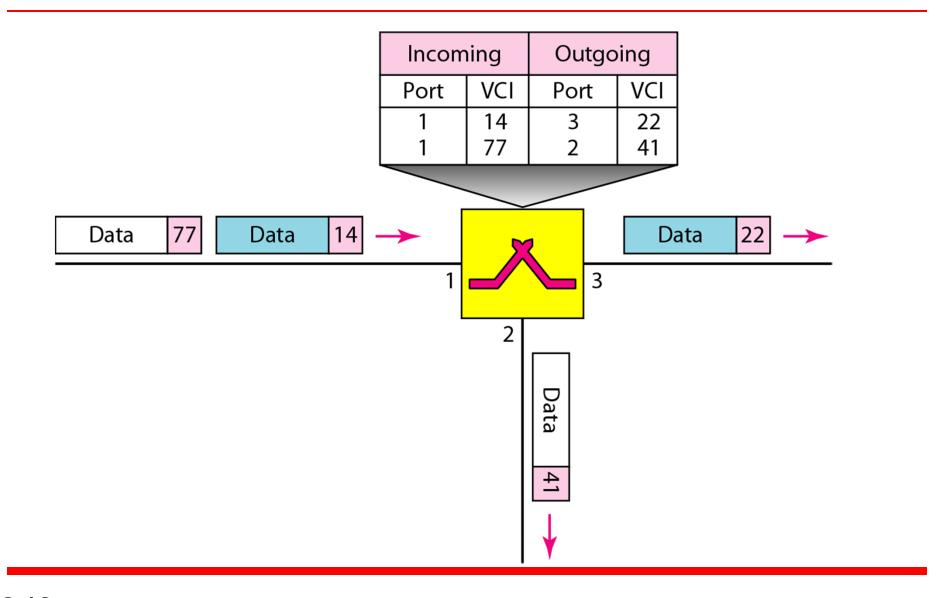
Figure 8.13 Source-to-destination data transfer in a virtual-circuit network
