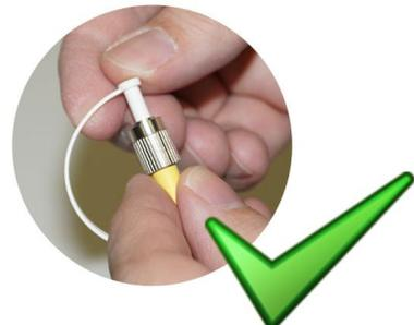
**IMPROPER ALIGNMENT OF THE KEY AND KEYWAY IS THE NUMBER ONE CAUSE OF POOR CONNECTIONS!**
