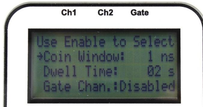
Use the up and down arrows on the coincidence counter to move the arrow to the "Coin Window" line. Once there, press the "SELECT" button on the coincidence counter. Use the up and down arrows to select and set the coincidence window to "1 ns" on the menu display. To accept this value, press the "SELECT" button again on the coincidence counter. Perform a similar operation for the "Dwell Time" line and set it to "02 s". When finished, press the menu button again to return to the startup screen.
