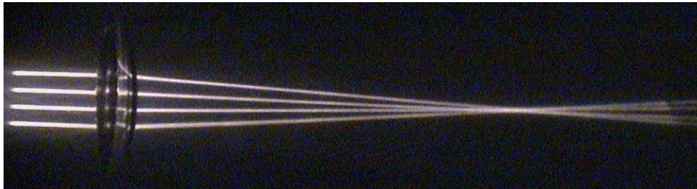
Fig. 2 Light focusing by a thin positive lens
