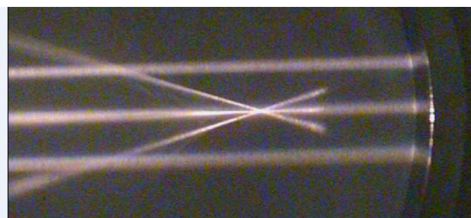
Fig. 1 Light focusing by a spherical surface
