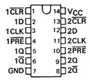
SN5473, SN54LS73A . . . J OR W PACKAGE SN7473 . . . N PACKAGE SN74LS73A . . . D OR N PACKAGE (TOP VIEW)
