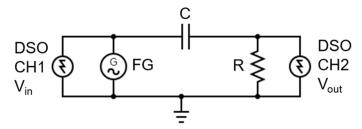
Using the oscilloscope, determine the ratio of the peak-to-peak amplitudes of the input and output voltages  $V_{\text{out}}/V_{\text{in}}$  as you did for the low pass filter. As you do these measurements, also measure the phase difference between  $V_{\text{out}}$  and  $V_{\text{in}}$  for each frequency.
