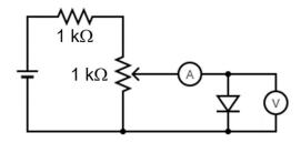
Reverse the diode and take data for the reverse direction. You may need the  $\mu A$  range for measuring the current. **Don't exceed 5 V** for the reverse measurement. Record V and I with a negative sign.
