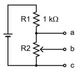
Using a DMM as an ohmmeter, identify which terminal of the potentiometer ("pot") is associated with the movable node b. Label the terminals so that a <u>clockwise</u> rotation of the shaft (when viewed against the end of the shaft) moves b from c toward a (so that the resistance across b and c is increasing).
