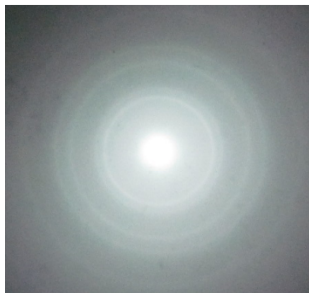
Fig. 11 The diffraction pattern from polycrystalline aluminum
