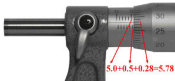
A typical micrometer screw gauge
